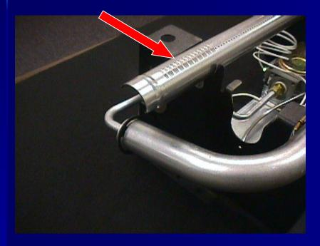
Clean the burner ports very well to remove any build up of dust and particles
