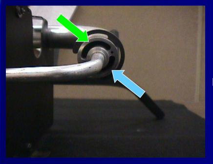
Use compressed air on both the upper and lower set of Air Injector Holes
